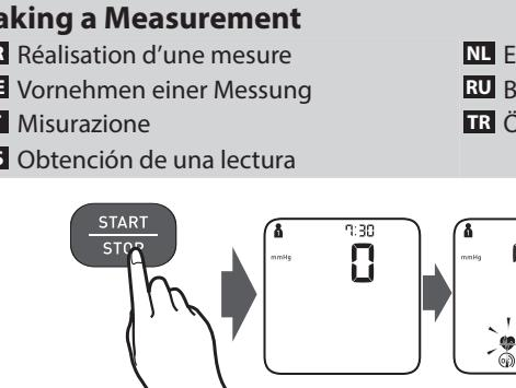
When the [START/STOP] button is pressed, the measurement is taken and saved automatically.
